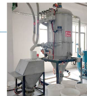
负压电子秤用于主料计量 Negative Pressure Electronic Scale
