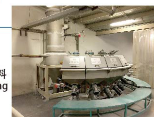
负压电子秤用于主料计量 Negative Pressure Electronic Scale
